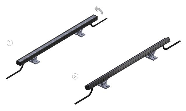
2. Screw in the screws through the screw holes on the tiltable stands.
