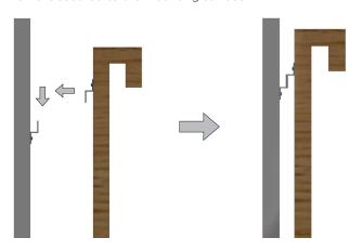
5. Use felt or other non-damaging shim material to fill any gaps between the frame and backlyte to keep it secure.
