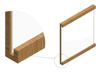
3. Make sure to enclose the custom frame to ensure the backlyte stays in place. Installation complete.
