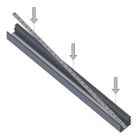
10. Attach lens onto fixture.
