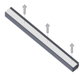
3. Screw the mounting clips onto the wall. Use a leveling tool to make sure the mounting clips are leveled.
