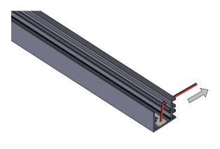
11. Attach end caps onto fixture with screws.
