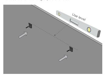
5. Drill a hole at the marked drill point on wall and match the hole in the wall with the hole on the back of fixture.
