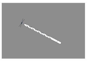
2. Drill a hole on the back of Channel close to the end for back-feed power wires to go through.
