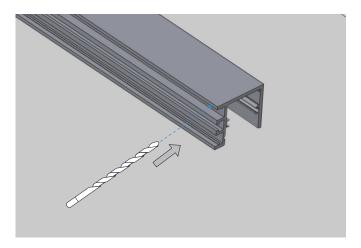
4. Mark drill point on wall through the back-feed power wire hole from fixture.
