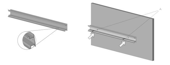
2. Insert Ribbonlyte (B) and make all necessary electrical connections (C).
