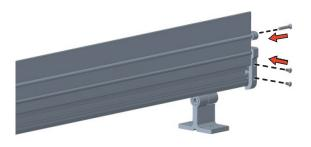
6. Tighten/loosen the flathead screws and rotate the Glare Shield until it is set at the desired angle.
