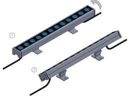
2. Secure the fixture in place by fastening the screws through the screw holes on one side of the tiltable stand.
