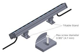
3. Rotate the fixture in the opposite direction and fasten the screws on the other side of the tiltable stand.
