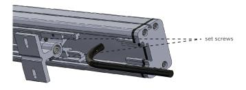
5. Secure the fixture on the pair of extension arms by fastening the screws in the tiltable stand to the extension arms. (See Step 1-4 for reference)
