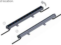
3. Tilt the fixture top to the other side and fasten screws through second set of screw holes on the tiltable stands (same as Step 2).
