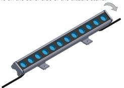
2. Secure the fixture in place by fastening the screws through the screw holes on one side of the tiltable stand.
