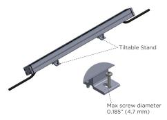
4. Connect to power supply and to additional fixture if desire to complete the installation.
