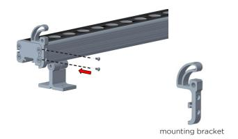
4. Put the copper standoff through the lower screw hole on the mounting bracket. Fasten the flathead screw through the top slot in the mounting bracket into the Glare Shield.
