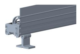
6. Tighten/loosen the flathead screws and rotate the Glare Shield until it is set at the desired angle.
