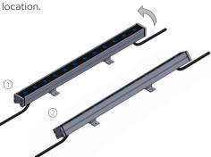
2. Fasten screws through the screw holes on the tiltable stands.
