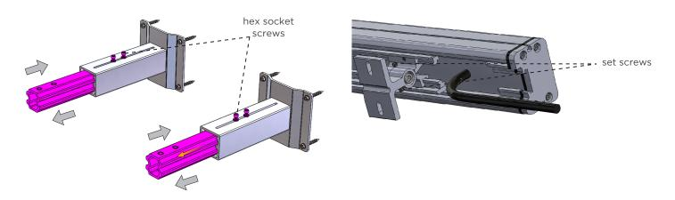
5. Secure the fixture on the pair of extension arms by fastening the screws in the tiltable stand to the extension arms. (See Step 1-4 for reference)
