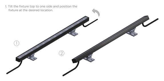
2. Screw in the screws through the screw holes on the tiltable stands.
