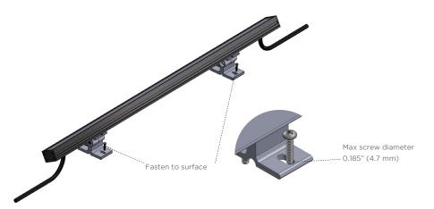
3. Tilt the fixture top to the other side and screw in the screws through the screw holes on the tiltable stands same as Step 2.
