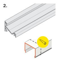
Cut channel and lens to desired (equal) lengths.
