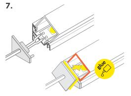
Attach end caps. For raised square lens, affix matching lens cap with glue. Fixture installation complete.
