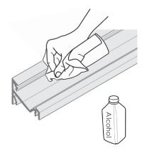
Clean the inside surface of the channel of dust and debris with rubbing alcohol. Dry.
