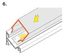
Attach lens by sliding or snapping into place.
