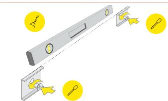
Check intended angle of fixture display. Measure and mark the desired location of the corner mounting clips. Drill a pilot hole for mounting clip fasteners. Screw the fasteners through the mounting clips to fix them in place on the surface.
