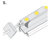
Apply RibbonLyte. Make all necessary electrical connections.
