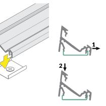
Align the channel above the mounting clips and push down to snap into place.
