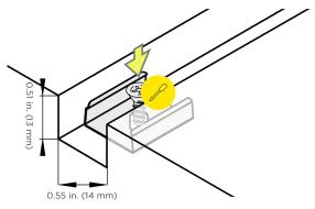
Measure and mark the desired location of the mounting clips. Drill a pilot hole for mounting clip fasteners. Screw the fasteners through the mounting clips to fix them in place on the surface.
