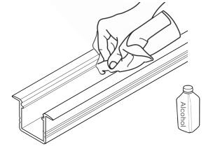
Clean the inside surface of the channel of dust and debris with rubbing alcohol. Dry.
