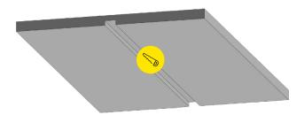
Measure the size of the channel and mounting clips and cut a recess into the surface to match the size of the channel and mounting clips.
