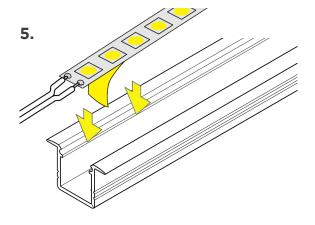
Apply RibbonLyte. Make all necessary electrical connections.
