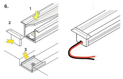
Attach lens by sliding or snapping into place. Attach end caps. Align the channel above the mounting clips and push down to snap into place. Fixture installation complete.
