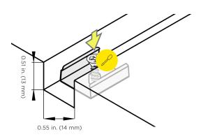
Measure and mark the desired location of the mounting clips. Drill a
