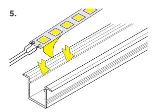
Apply RibbonLyte. Make all necessary electrical connections.
