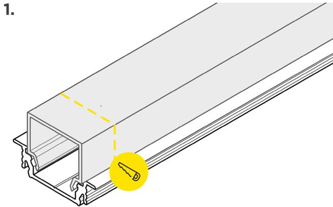
Cut channel and lens to desired length.
