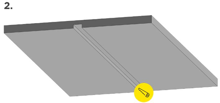
Measure the size of the channel and mounting clips and cut a recess into the surface to match the size of the channel and mounting clips.
