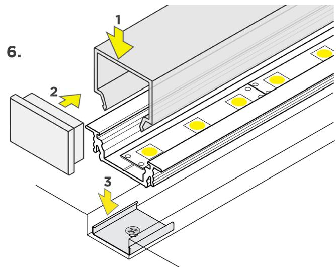
Attach lens by sliding or snapping into place. Attach end caps. Align the channel above the mounting clips and push down to snap into place. Fixture installation complete.
