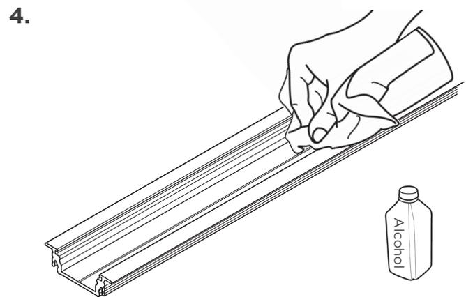
Clean the inside surface of the channel of dust and debris with rubbing alcohol. Dry.
