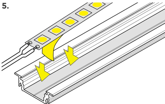
Apply RibbonLyte. Make all necessary electrical connections. (Feed through end caps as needed.)
