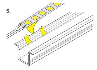
Apply RibbonLyte. Make all necessary electrical connections.
