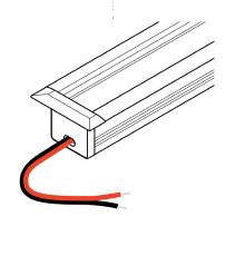
Attach lens by sliding or snapping into place. Attach end caps. Align the channel above the mounting clips and push down to snap into place. Fixture installation complete.
