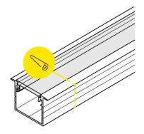
Cut channel and lens to desired length.
