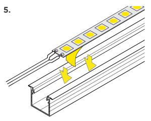
Apply RibbonLyte. Make all necessary electrical connections. (Feed through end caps as needed.)
