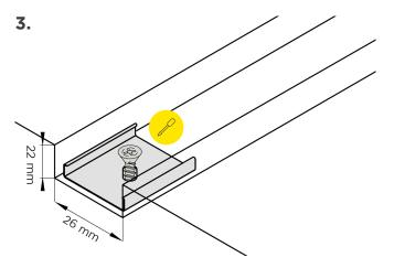
Screw the fasteners through the mounting clips to fix them in place on the surface.
