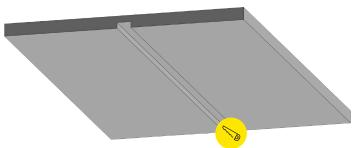
Measure the size of the channel and mounting clips and cut a recess into the surface to match the size of the channel and mounting clips.
