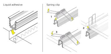
**NOTE:** If mounting clips cannot be used, apply a liquid adhesive in the recess before placing the channel OR attach spring clips to channel, push channel through recess and deploy spring clips.
