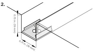
Screw the fasteners through the mounting clips to fix them in place on the recessed surface.
