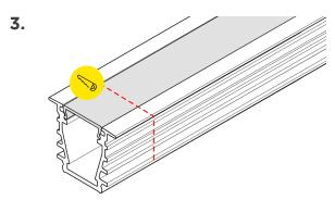
Cut channel and lens to desired (matching) length.
