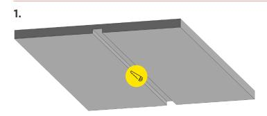
Measure the size of the channel and mounting clips and cut a recess into the surface to match the size of the channel. Note that end caps will increase the length of channel where applied.
