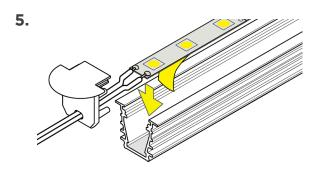
Apply RibbonLyte. Make all necessary electrical connections.
