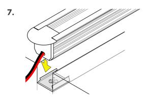
Align the channel above the mounting clips and push down to snap into place. Fixture installation complete.
