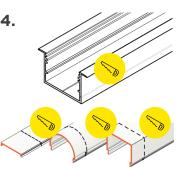
Cut channel and lens to desired (equal) lengths.
