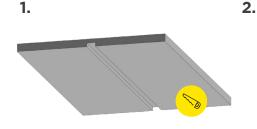
Measure the size of the channel and mounting clips and cut a recess into the surface to match the size of the channel. (Recommended width of 38 mm and depth of 25 mm.)
