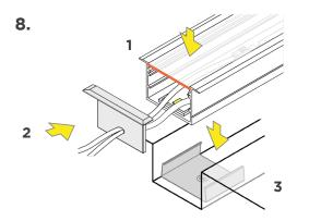
Attach lens by sliding or snapping into place. Attach end caps. Align the channel above the mounting clips & push down to snap into place.
