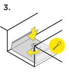
Screw the fasteners through the mounting clips to fix them in place on the surface.
