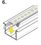
Apply RibbonLyte. Make all necessary electrical connections.
