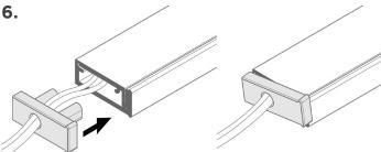
Attach lens by snapping "lid" into place.
