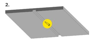
Measure the size of the channel and cut a recess into the surface to match the size of the channel. \*Note: Add 1 mm per meter of the fixture to the mounting space to accommodate minor expansion when using higher wattages.
