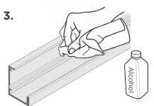
This fixture opens like a case, with the mounting surface inside the "lid." Do not close "lid" until instructed. Clean the inside surface of the channel of dust and debris with rubbing alcohol. Dry.
