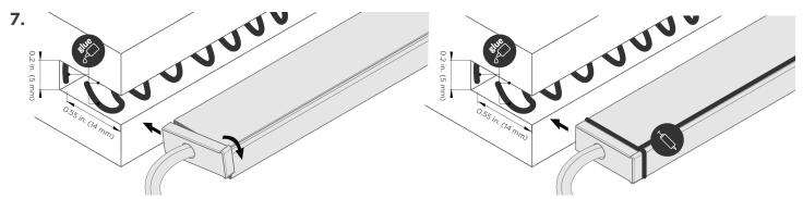
Apply glue to bottom and back of recessed surface. In areas of high humidity, secure connections with silicone. Tighten end cap and insert into recessed surface. Fixture installation complete.
