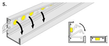
Attach lens by snapping "lid" into place.
