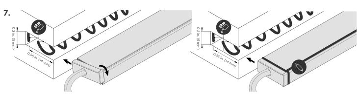
Apply glue to bottom and back of recessed surface. In areas of high humidity, secure connections with silicone. Tighten end cap and insert into recessed surface. Fixture installation complete.
