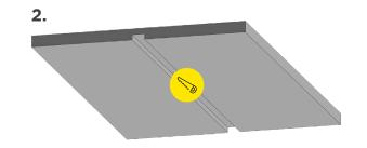
Pre-drill holes in the end caps for wire pass through. Measure the size of the channel and cut a recess into the surface to match the size of the channel. \*Note: Add 1 mm per meter of the fixture to the mounting space to accommodate minor expansion when using higher wattages.
