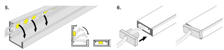
Attach lens by snapping "lid" into place.
