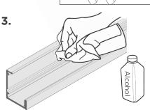
This fixture opens like a case, with the mounting surface inside the "lid." Do not close "lid" until instructed. Clean the inside surface of the channel of dust and debris with rubbing alcohol. Dry.
