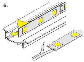
Apply RibbonLyte. Make all necessary electrical connections.
