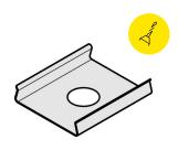
Pre-drill holes in mounting clips for fasteners.
