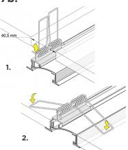
If mounting clips cannot be used, attach spring clips to channel, push channel through recess and deploy spring clips.
