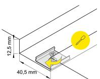
Screw the fasteners through the mounting clips to fix them in place on the recessed surface.
