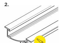
Cut channel and lens to desired fit, noting that lens will be longer than channel where end caps are used.
