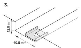
Measure the size of the channel and mounting clips and cut a recess into the surface to match the size of the channel (approx. 12.5 mm deep, 40.5 mm wide). Note that end caps will increase the length of channel where applied.
