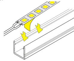
Apply RibbonLyte and make all necessary electrical connections. (Run through end caps as needed.)
