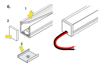
Attach lens by sliding or snapping into place. Attach end caps. Align the channel above the mounting clips and push down to snap into place. Fixture installation complete.
