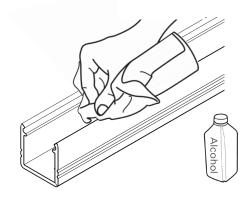
Clean the inside surface of the channel of dust and debris with rubbing alcohol. Dry.
