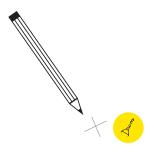
Measure and mark the desired location of the corner mounting clips. Drill a pilot hole for mounting clip fasteners.
