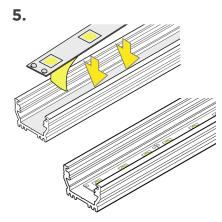
Apply RibbonLyte. Make all necessary electrical connections.
