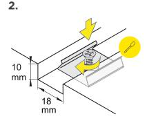
Screw the fasteners through the mounting clips to fix them in place on the surface.
