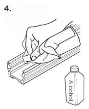
Clean the inside surface of the channel of dust and debris with rubbing alcohol. Dry.
