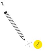
Measure and mark the desired location of the mounting clips. Drill a pilot hole for mounting clip fasteners.
