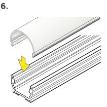
Attach lens by sliding or snapping into place.
