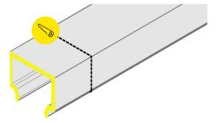
Cut channel and lens to desired (equal) lengths.
