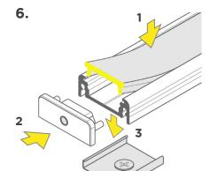
Attach lens by sliding or snapping into place. Attach end caps. See next step for mounting clip instruction.
