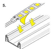
Apply RibbonLyte and make all necessary electrical connections. (Run through end caps as needed.)
