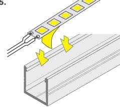
Apply RibbonLyte and make all necessary electrical connections. (Run through end caps as needed.)
