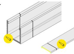
Cut channel and lens to desired (equal) lengths.
