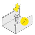
Screw the fasteners through the mounting clips to fix them in place on the surface.
