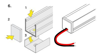
Attach lens by sliding or snapping into place. Attach end caps. Align the channel above the mounting clips and push down to snap into place. Fixture installation complete.
