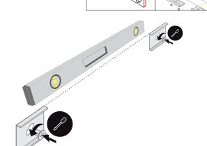
Measure and mark the desired location of the mounting clips. Drill a pilot hole for mounting clip fasteners. Screw the fasteners through the mounting clips to fix them in place on the surface.
