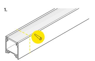
Cut channel and lens to desired length.
