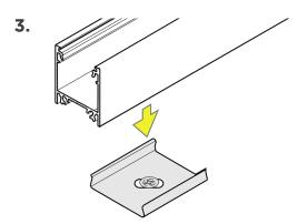
Align the channel above the mounting clips and push down to snap into place.
