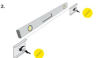
Measure and mark the desired location of the mounting clips. Drill a pilot hole for mounting clip fasteners. Screw the fasteners through the mounting clips to fix them in place on the surface.
