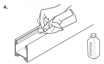
Clean the inside surface of the channel of dust and debris with rubbing alcohol. Dry.
