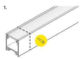
Cut channel and lens to desired length.
