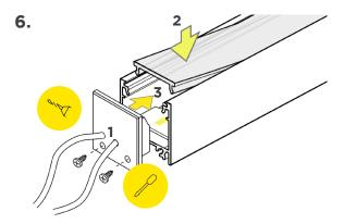
Drill hole in end caps for electrical connections. Feed wire through and make all necessary electrical connections. Attach lens by sliding or snapping into place. Attach end caps. Fixture installation complete.
