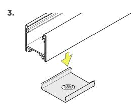
Align the channel above the mounting clips and push down to snap into place.
