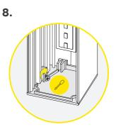
Insert the end caps and secure with the screws provided.
