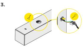
Drill any holes in channel needed for back-feed electrical connections.
