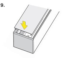
Attach the lens by snapping into place. Installation complete.
