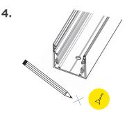
Mark location of holes on mounting surface. Drill pilot holes in mounting surface.
