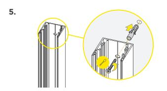
Align channel to pilot holes and attach with screws. Be sure to pull through any wires needed for back-feed electrical connection.
