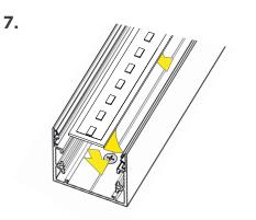
Apply RibbonLyte to mounting surface and make all necessary electrical connections.
