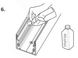
Clean the channel mounting surface of dust and debris using a cloth and rubbing alcohol. Dry.
