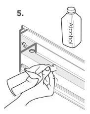
Clean the inside surface of the channel of dust and debris with rubbing alcohol. Dry.
