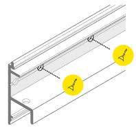
Pre-drill holes along back of fixture for mounting.
