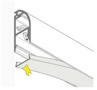
Attach lens by sliding or snapping into place.
