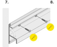
Mount fixture by screwing through middle of channel mounting section as needed.
