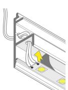
Apply RibbonLyte. Make all necessary electrical connections.
