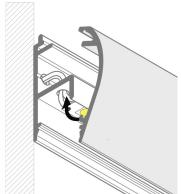
Install large cover to front of channel. Hook cover to bottom lip of channel, then click carefully into top lip. \*Note: DO NOT try to remove large cover by force. Carefully lift top lip and pull back to remove cover (from the top out toward you).
