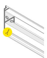
Drill holes in top of ribbon channel and back of fixture for wiring power supply.
