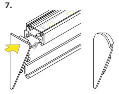
Attach end caps if needed. If using raised round lens, use rounded end cap (right).
