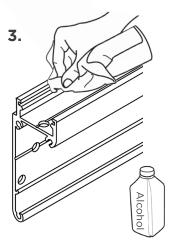
Clean the inside surface of the channel of dust and debris with rubbing alcohol. Dry.
