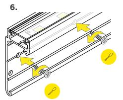
Mount fixture by screwing through middle of channel mounting section.
