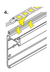
Apply RibbonLyte. Make all necessary electrical connections.
