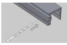
5. Drill a hole at the marked drill point on wall and match the hole in the wall with the hole on the back of fixture.
