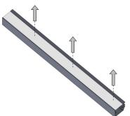
4. Mark drill point on wall through the back-feed power wire hole from fixture.
