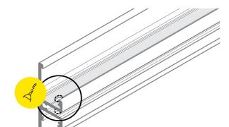
Drill holes in inside channel beds for electrical connections.
