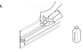
Clean the inside surfaces of the channel of dust and debris with rubbing alcohol. Dry.
