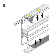
Apply RibbonLyte to appropriate channel beds. Make all necessary electrical connections.
