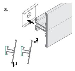
Align the channel above the mounting clips and push down to snap into place.
