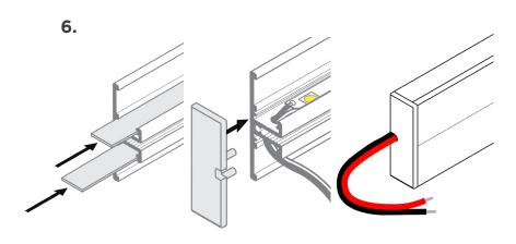
Attach lens by sliding or snapping into place. Attach end caps to complete installation.
