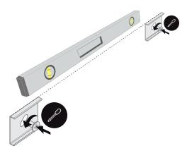
Measure and mark the desired location of the mounting clips. Drill a pilot hole for mounting clip fasteners. Screw the fasteners through the mounting clips to fix them in place on the surface.
