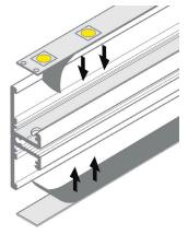
Apply RibbonLyte to appropriate channel beds. Make all necessary electrical connections.
