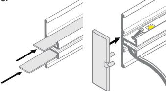
Attach lens by sliding or snapping into place. Attach end caps to complete installation.
