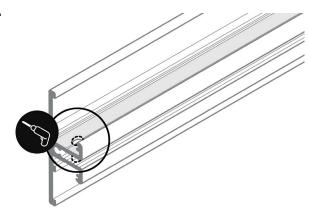
Drill holes in inside channel beds for electrical connections.
