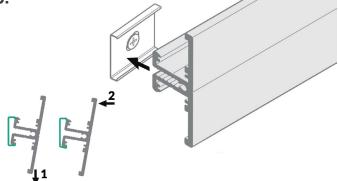
Align the channel above the mounting clips and push down to snap into place.
