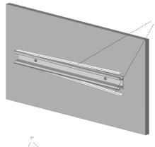
4/5. Place the front cover (E) over the mounted wall fixture and fasten both end caps (F) to the front cover with screws.
