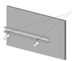
2/3. Insert RibbonLyte (B) and make all necessary electrical connections (C). Attach lenses (D).
