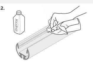
Clean the inside surface of the channel of dust and debris with rubbing alcohol. Dry.
