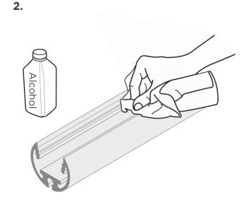
Clean the inside surface of the channel of dust and debris with rubbing alcohol. Dry.
