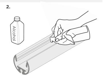
Clean the inside surface of the channel of dust and debris with rubbing alcohol. Dry.
