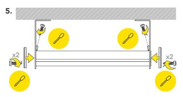
Slide fixture through mounting arm and attach end caps from outside of each extension arm. Fixture installation complete.
