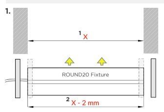
Measure and align wall mounts. Cut channel and lens to equal lengths, 2 mm less than distance between mounting surfaces.
