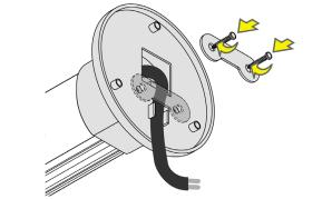
Attach ring holder to each end. Secure wires by attaching small metal plate on each end.
