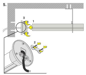
Attach fixture to side holder, and then secure wires by attaching small metal plate on each end. Secure side holder to wall with fasteners.
