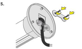
Attach side holder to each end. Secure wires by attaching small metal plate on each end.
