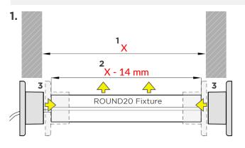
Measure and align wall mounts. Cut channel and lens to equal lengths, 14 mm less than distance between mounting surfaces.
