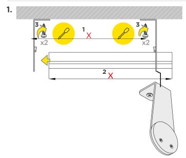
Measure, align and mark spots to attach extension arms to ceiling. Cut channel and lens to desired (equal) lengths. Secure extension arms to ceiling with fasteners.
