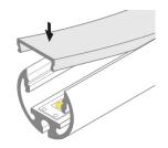
2. Clean the inside surface of the channel of dust and debris with rubbing alcohol. Dry.
