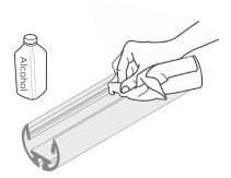
2. Clean the inside surface of the channel of dust and debris with rubbing alcohol. Dry.
