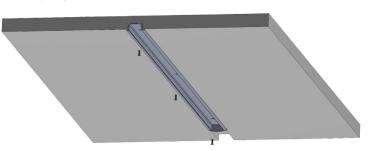
Clean the inside of the channel free of dirt and debris with rubbing alcohol and then place the ribbonlyte inside of the channel. Make all necessary electrical connections.
