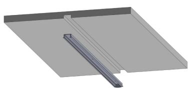
2. Place the channel into the recess so that it fits snug with the flanges over the lip of the surface.
