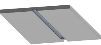
3. Secure the fixture into place with the fasteners. If fasteners cannot be used then a liquid adhesive can be used in the recess before placing the channel.
