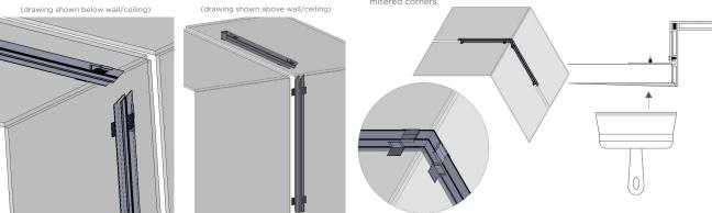
6. Connect Light Engine Assembly (Part B) to power. Fit Light Engine Assembly into Recessed Assembly (Part A).
