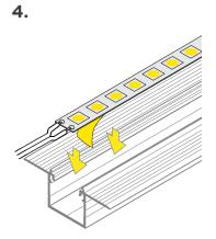
Apply RibbonLyte. Make all necessary electrical connections. (Feed through end caps as needed.)
