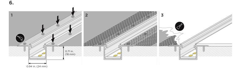
Place fixture in recess and attach by screwing flanges to surface. Mud-in to achieve flush finish. Fixture installation complete.
