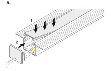
Attach lens by sliding or snapping into place. Attach end caps.
