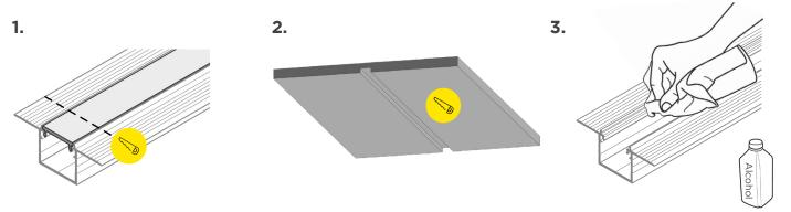
Cut channel and lens to desired length.
