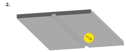
Cut channel and lens to desired length.
