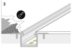
Place fixture in recess and attach by screwing flanges to surface. Mud-in to achieve flush finish. Fixture installation complete.
