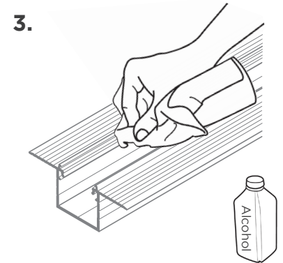
Clean the inside surface of the channel of dust and debris with rubbing alcohol. Dry.
