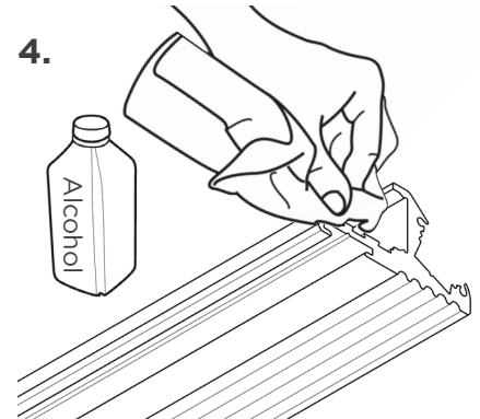
4. Clean the bottom RibbonLyte mounting surface in the channel of dust and debris with rubbing alcohol. Dry.
