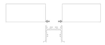
3. Slide the spring clips through the slot on the top of the channel and then fasten in place with the set screws.
