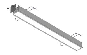
6. Pull the springs together on the spring clips and feed the fixture through the ceiling so the spring clips sit flush on the hidden surface of the drywall.
