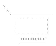
2. Place Flexible BackLyte in desired location. Screw through the screw holes on Flexible BackLyte to secure it in place.
