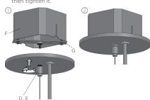
2. Attach the Cross Bar (G) to the Junction Box (F) with screws, & insert the screw into the hole in the center of the Cross Bar (G).
