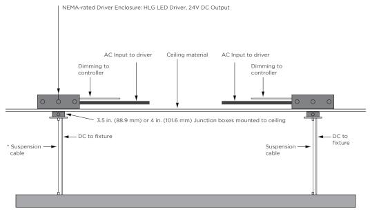
$<sup>^{\</sup>ast}$  Max Suspension Cable length from ceiling to fixture: 150 in. (3.81 m)
