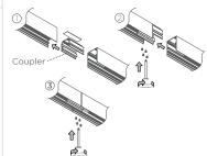
4. Reverse Step 1 and 2 to reattach the reflectors with LEDs on the fixture, and then reattach the lenses to finish.
