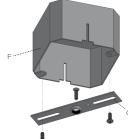
4. Put the screw in the center of the Cross Bar (G) on the Junction Box (F) through the Coupler Top and Base (D, E) and then tighten it.
