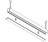
2. Remove the reflector with LEDs.
