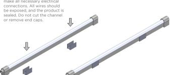
3. Push the Neon Contour Plus into place in the mounting channel and make all necessary electrical connections. All wires should be exposed, and the product is sealed. Do not cut the channel or remove end caps.
