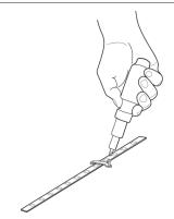
5. Tighten the screws through the silicone pads until RibbonLyte is tightly secured.
