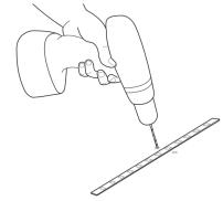
4. Drill pilot holes at center of each mark.
