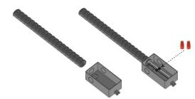
4. Mark the desired location of the Rigid AC on the mounting surface. Drill pilot holes for the mounting clips and then fasten the mounting clips to the surface with screws.
